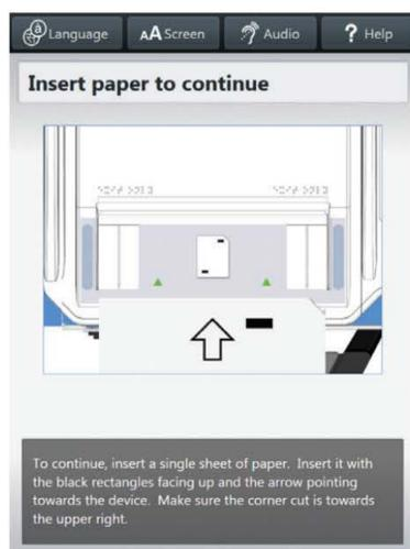
To continue, insert a single sheet of paper. Insert it with the black rectangles facing up and the arrow pointing towards the device. Make sure the corner cut is towards the upper right.
